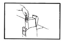
3. The entire sealed cassette is then easily removed from Counter Cache II, and an empty cassette replaces it.
