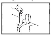
2. To change the cassette in Counter Cache II, the box is opened with a key. The locked-in cassette can only be removed by inserting a separate plastic key plate (as shown), which both seals and releases the
